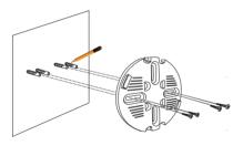
Figure 3: Attaching the Mounting Plate
