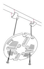
Figure 6: Attaching the Mounting Plate
